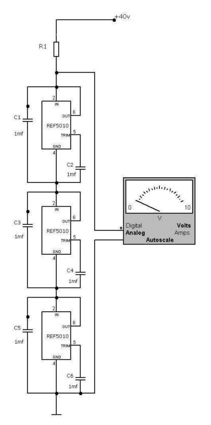
Figure 2. REF5010 Connected Serially as Usual Zener Diodes
