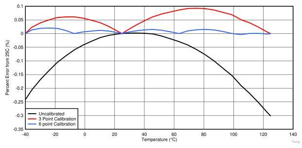
Figure 5-1. Temperature Drift Error With Calibration Profiles
