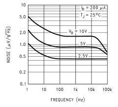
Figure 6-1. LM4050 Noise Voltage vs Frequency
