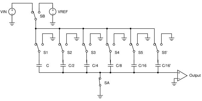
Figure 7-1. SAR ADC Sampling Architecture
