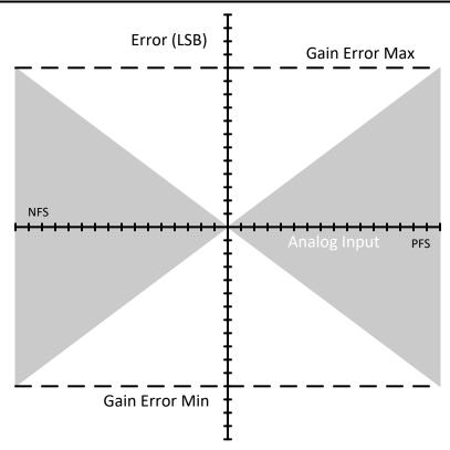
Figure 4-2. ADC Gain Error
