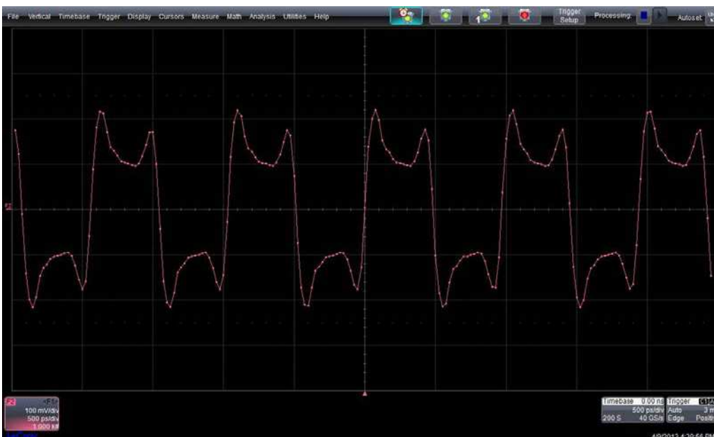
Figure 15. Pre Cursor & Post Cursor Taps Applied to Channel & Linear Equalizer with 3.5dB of Loss
