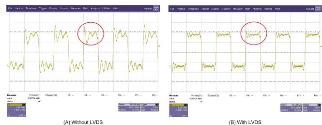
Figure 3. AMC1305 ADC Output Voltage Waveform with and without LVDS
