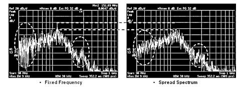
Figure 6. Comparison of Fixed-Frequency and Spread-Spectrum Modulation
