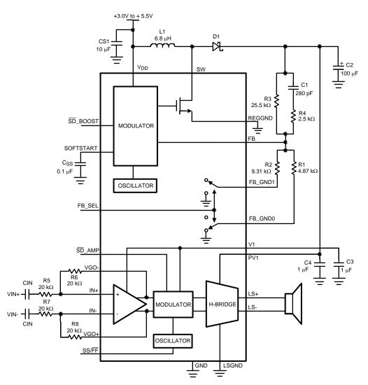
Figure 7. LM48511 - A Spread-Spectrum Modulated Class D Amplifier
