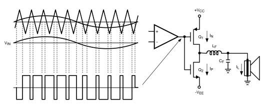
Figure 4. The Class D Audio Amplifier PWM
