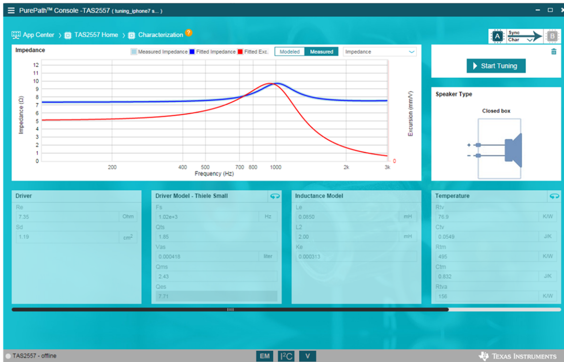
Figure 6. Impedance and Excursion Characterization Result with PPC3 and LB2
