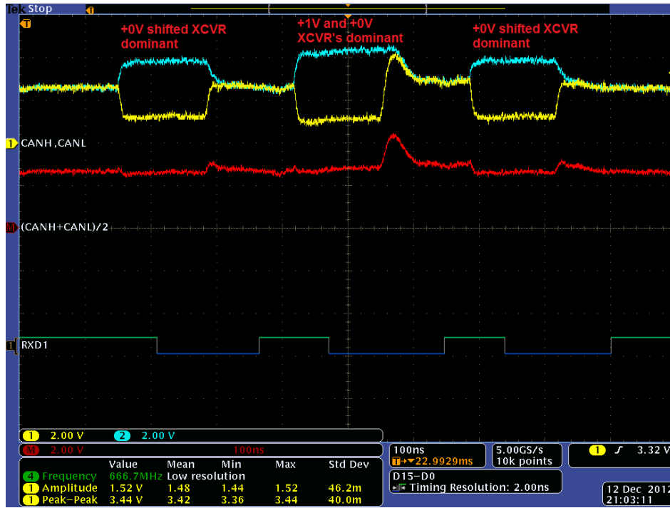
Figure 5. Waveform of Two SN65HVD255 Transceivers, One with a +1V Ground Shift
