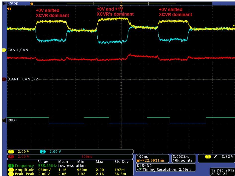
Figure 6. Waveform of Two 5V SN65HVD255 Transceivers with Split Termination, One with a +1V Ground Shift
