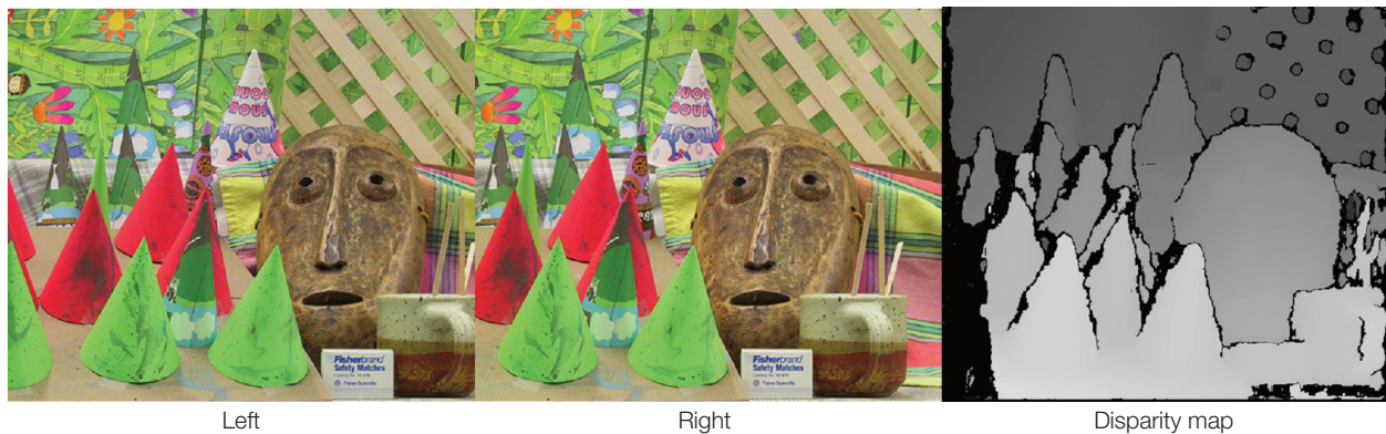
Figure 11: Cones and faces from Middlebury dataset. The disparity calculation is performed using simple SAD. The disparity keeps changing marginally on the curved surfaces, while it changes drastically on the object boundaries. See the disparity holes in the fence on the top-right, other object discontinuities and occlusions on left border.
