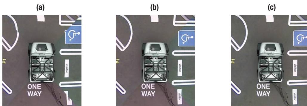
Figure 19: The composite surround view synthesized from four fish-eye frames shown in Figure 1: (a), without proper geometric alignment or photometric alignment; (b), with proper geometric alignment, but without photometric alignment, and (c), with our proposed geometric and photometric alignment algorithms. Without geometric alignment, misalignment at view boundaries is very noticeable. Without photometric alignment, the stitched surround view output suffers color and brightness inconsistency at stitching boundaries. In (c), we achieve a high-quality seamlessly stitched result.
