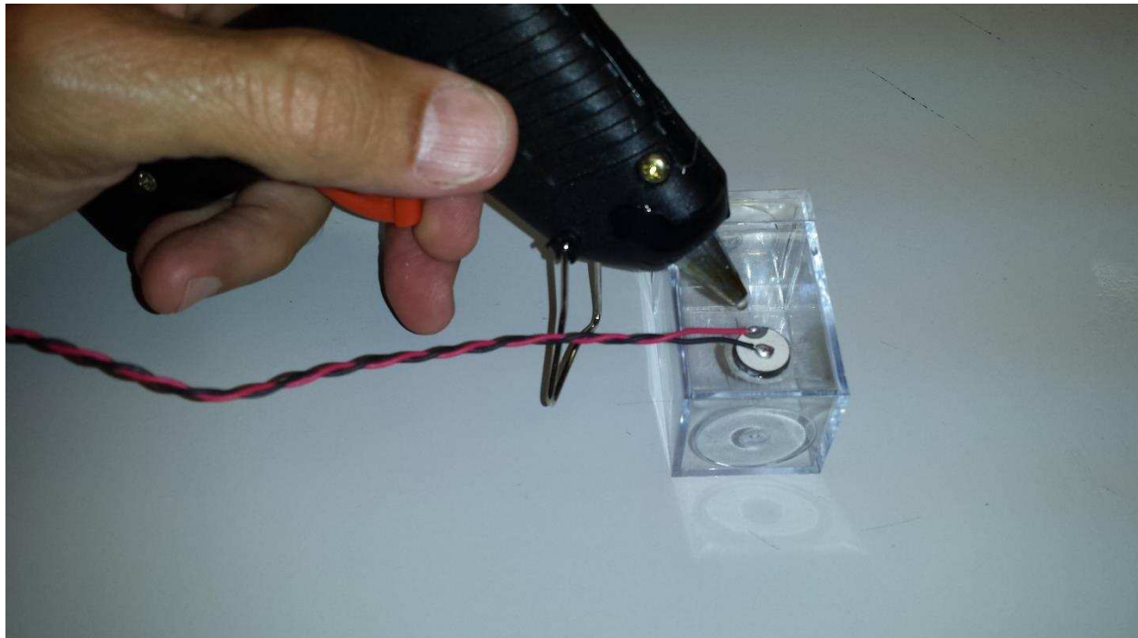
Figure 4. Applying Hot Glue to Transducer
