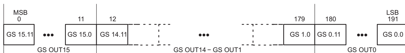
Figure 17. Grayscale Data Packet Format
