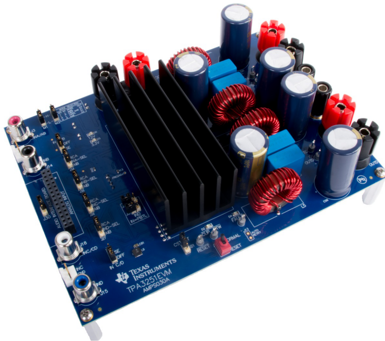
Figure 1. TPA3251 Evaluation Module
