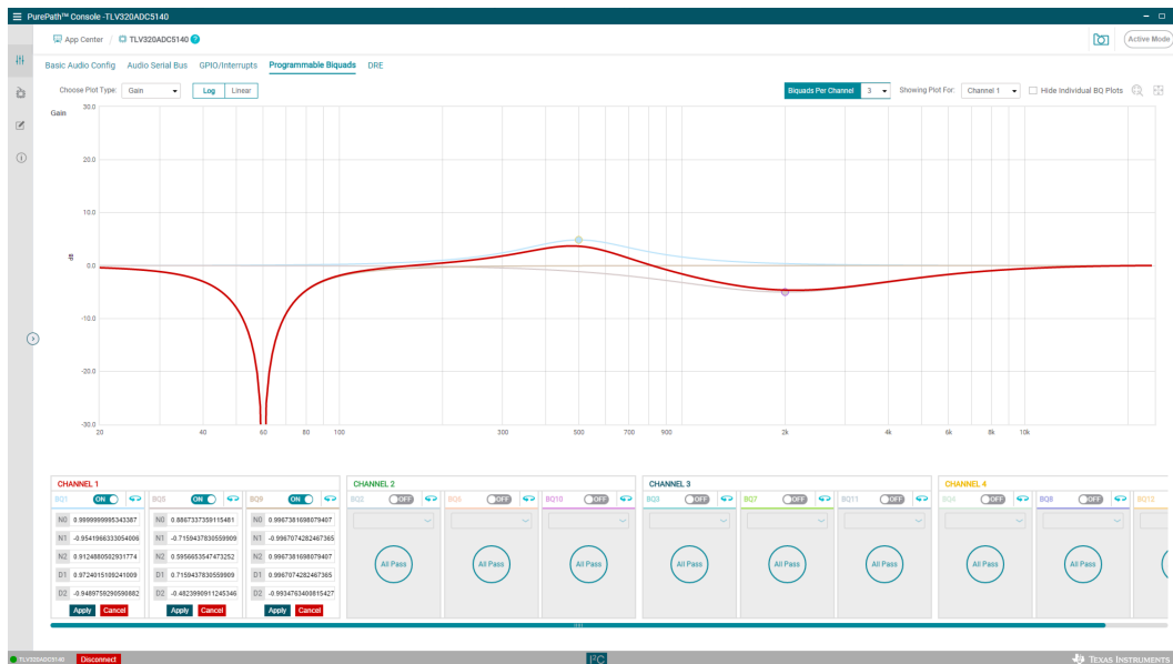
Figure 5. PurePath Console Programmable Biquad Filter Example Showing the Computed Coefficients in Normalized Floating Point Format
