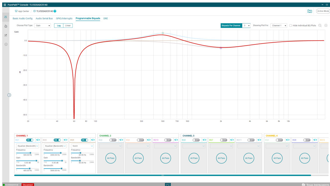
Figure 4. PurePath Console Programmable Biquad Filter Example
