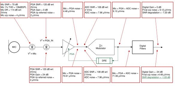
Figure 5-1. DRE Block Diagram
