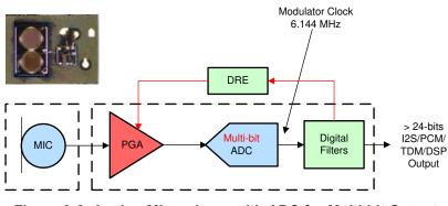
Figure 3-2. Analog Microphone with ADC for Multi-bit Output
