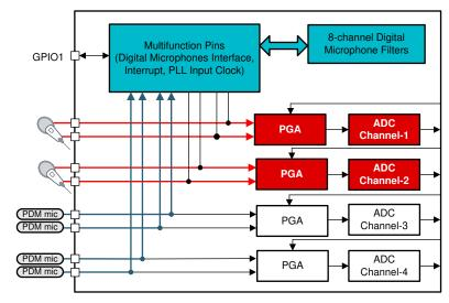
Figure 6-4. Combination Microphones System Block Diagram
