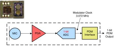
Figure 3-1. Digital PDM Microphone for 1-bit Output
