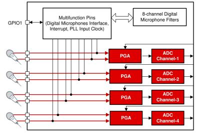
Figure 6-2. Analog Microphones System Block Diagram
