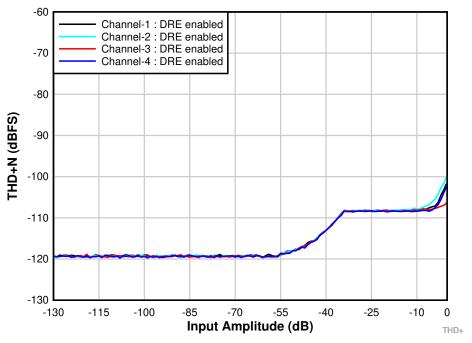
Figure 5-2. THD+N Performance Measurement with DRE Enabled
