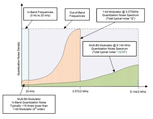
Figure 4-1. Quantization Noise Density
