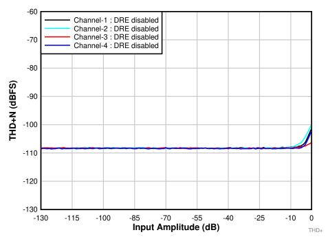
Figure 5-3. THD+N Performance Measurement with DRE Disabled
