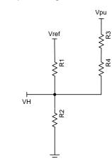
$$\frac{V_{PU} - V_{H}}{R_{3} + R_{4}} + \frac{V_{REF} - V_{H}}{R_{1}} = \frac{V_{H}}{R_{2}} \Rightarrow R_{1} = \frac{V_{REF} - V_{H}}{\frac{V_{H}}{R_{2}} - \frac{V_{PU} - V_{H}}{R_{2} + R_{4}}}$$
