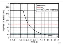
Figure 3. Magnetic Flux Density for Case Tamper Detection
