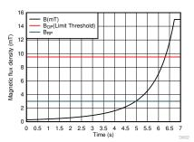
Figure 4. Magnetic Flux Density for End-of-Travel Detection
