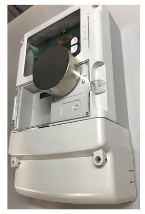
Figure 1. Magnetic Tampering in Electricity Meters
