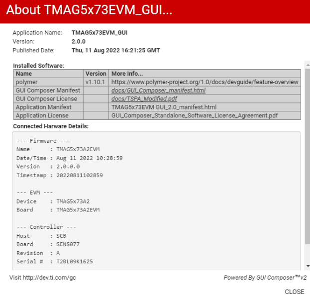
Figure 4-21. Firmware Revision Version in GUI About Screen
