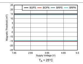
Figure 6-6. 15-mT Magnetic Threshold vs Supply
