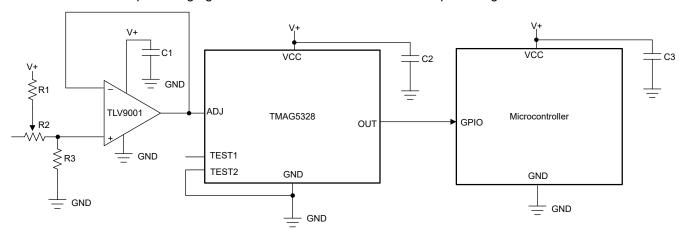
Figure 8-4. Setting BOP of One TMAG5328 Device Using a Voltage Divider and Potentiometer
