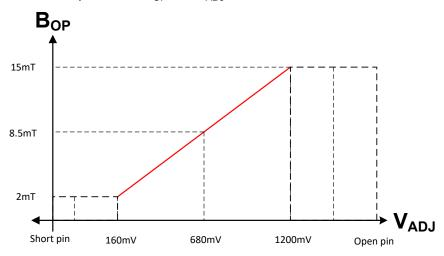
Figure 7-6. B<sub>OP</sub> vs R<sub>ADJ</sub>
