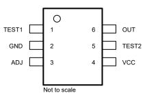
Figure 5-1. DBV Package 6-Pin SOT-23 Top View
