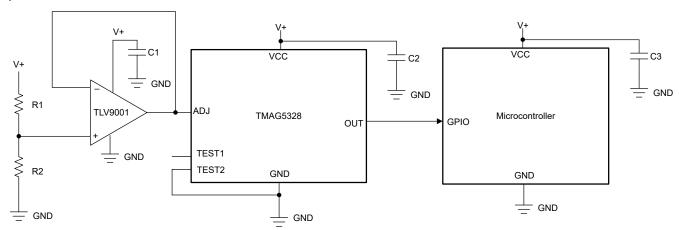
Figure 8-3. Setting B<sub>OP</sub> of One TMAG5328 Device Using a Voltage Divider
