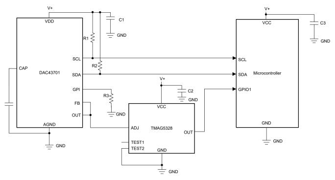
Figure 8-2. Setting B<sub>OP</sub> of One TMAG5328 Device Using a DAC
