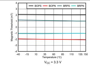
Figure 6-1. 2-mT Magnetic Threshold vs Temperature
