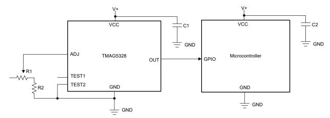
Figure 8-5. Setting B<sub>OP</sub> of One TMAG5328 Device Using a Potentiometer and the TMAG5328's Internal Current Source
