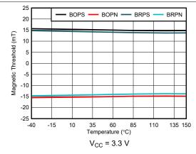
Figure 6-5. 15-mT Magnetic Threshold vs Temperature
