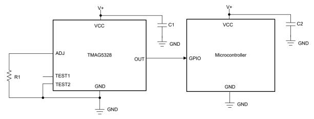
Figure 8-1. Setting B<sub>OP</sub> of One TMAG5328 Device Using a Resistor
