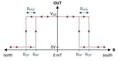
Figure 7-2. Omnipolar Functionality
