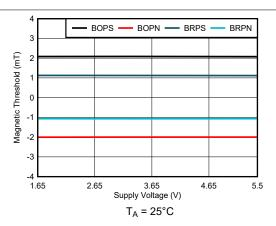
Figure 6-2. 2-mT Magnetic Threshold vs Supply
