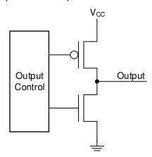
Figure 7-3. Push-Pull Output (Simplified)
