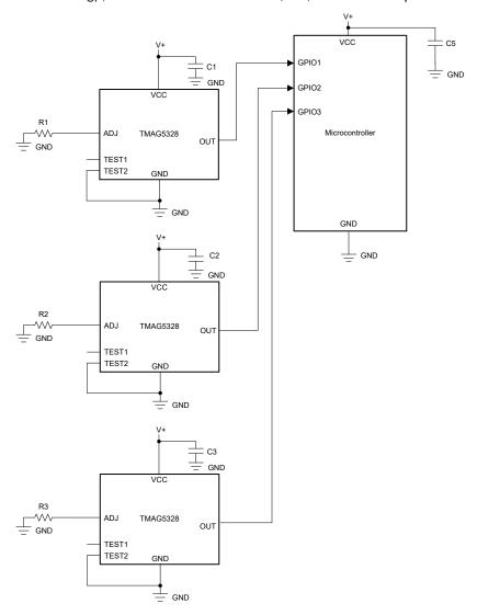
Figure 8-6. Setting B<sub>OP</sub> of Three TMAG5328 Devices Using Three Resistors
