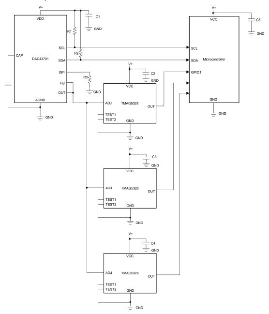
Figure 8-7. Setting B<sub>OP</sub> of Three TMAG5328 Devices Using a DAC
