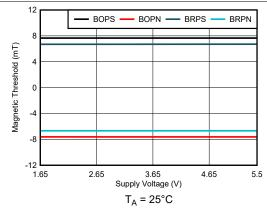
Figure 6-4. 7.5-mT Magnetic Threshold vs Supply
