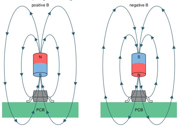
Figure 7-1. Flux Direction Polarity
