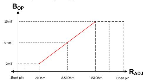
Figure 7-5. B<sub>OP</sub> vs R<sub>ADJ</sub>
