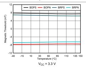
Figure 6-3. 7.5-mT Magnetic Threshold vs Temperature
