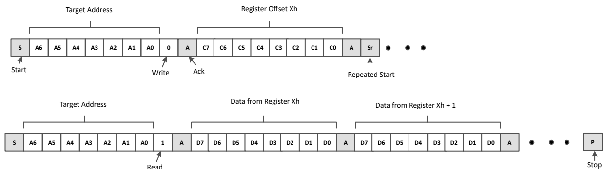
Figure 8-7. I2C Read with Repeated Start
