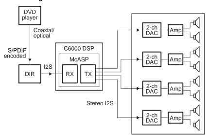
Figure 1-1. McASP to Parallel 2-Channel DACs
