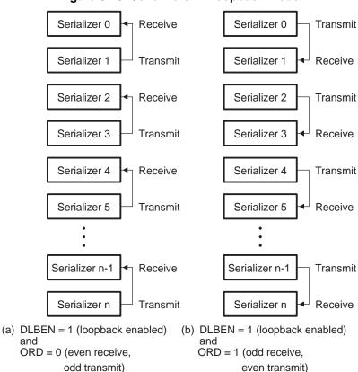
Figure 3-13. Serializers in Loopback Mode
