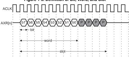
Figure 1-6. Definition of Bit, Word, and Slot
