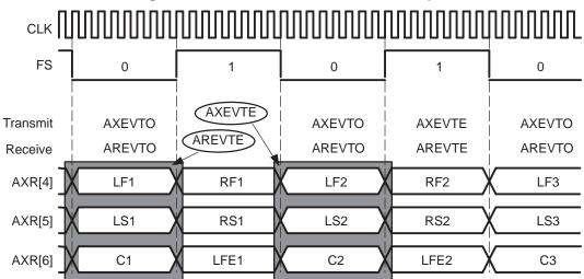
Figure 3-7. DMA Events in an Audio Example
