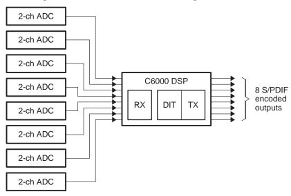
Figure 1-5. McASP as 16 Channel Digital Processor
