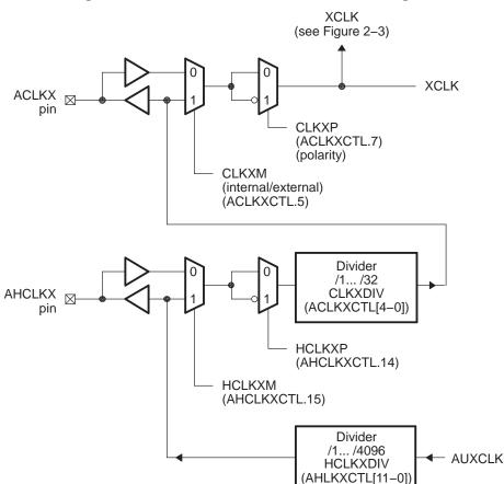
Figure 2-2. Transmit Clock Generator Block Diagram
