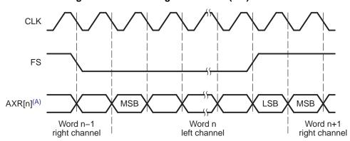
Figure 1-11. Inter-Integrated Sound (I2S) Format
