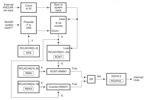
Figure 3-12. Receive Clock Failure Detection Circuit Block Diagram
