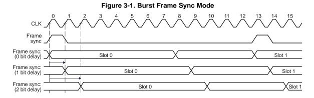
The control registers must be configured as follows for the burst transfer mode. The burst mode specific bit fields are in bold face:
