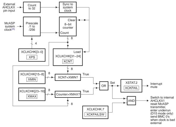
Figure 3-11. Transmit Clock Failure Detection Circuit Block Diagram
