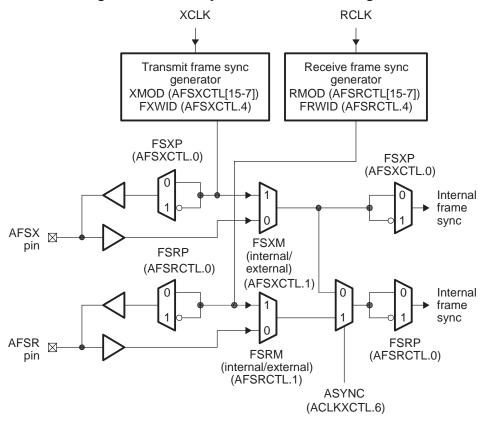
Figure 2-4. Frame Sync Generator Block Diagram
