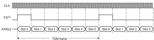
Figure 1-9. TDM Format-6 Channel TDM Example
