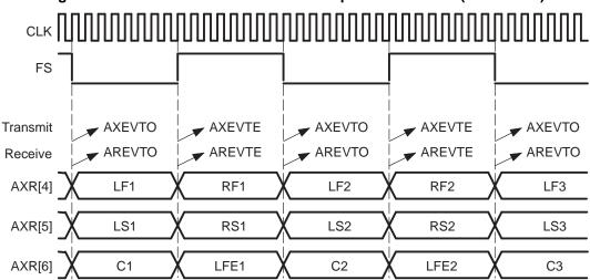
Figure 3-6. DMA Events in an Audio Example-Four Events (Scenario 2)
