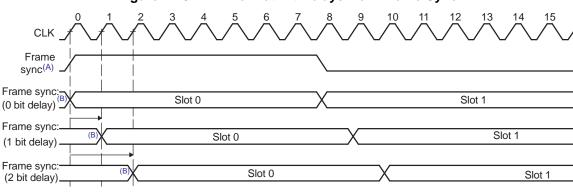
Figure 1-10. TDM Format Bit Delays from Frame Sync
