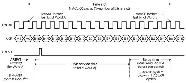
Figure 3-4. DSP Service Time Upon Receive DMA Event (AREVT)
