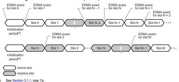
Figure 3-2. Transmit DMA Event (AXEVT) Generation in TDM Time Slots
