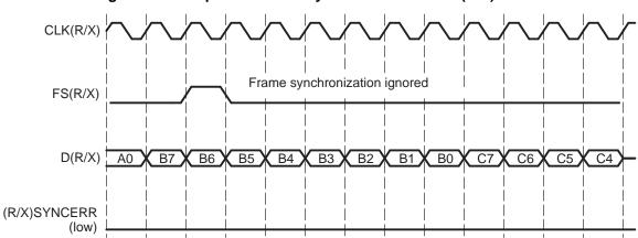
Figure 26. Unexpected Frame Synchronization With (R/X)FIG = 1
