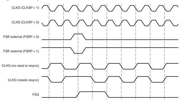
Figure 7. CLKG Synchronization and FSG Generation When GSYNC = 1 and CLKGDV = 1
