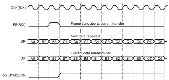
Figure 25. Unexpected Frame Synchronization With (R/X) FIG = 0
