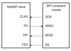
The clock stop mode (CLKSTP) of the McBSP provides compatibility with the SPI protocol. The McBSP supports two SPI transfer formats that are specified by the clock stop mode bits (CLKSTP) in SPCR. The CLKSTP bits in conjunction with the CLKXP bit in PCR allows serial clocks to be stopped between transfers using one of four possible timing variations, as shown in Table 16. Figure 50 and Figure 51 show the timing diagrams of the two SPI transfer formats and the four timing variations.
