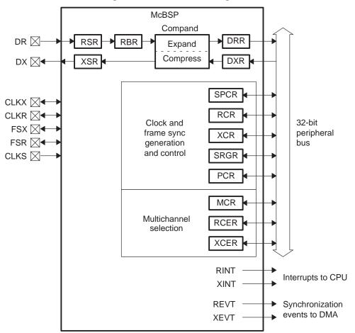
Figure 1. McBSP Block Diagram
