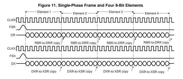
The example in Figure 11 can also be viewed as a data stream of a single-phase frame of one 32-bit data element, as shown in Figure 12. In this case:
