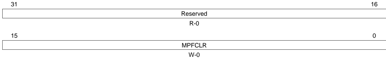
Figure 3-22. Memory Protection Fault Clear Register (L1DMPFCR)
