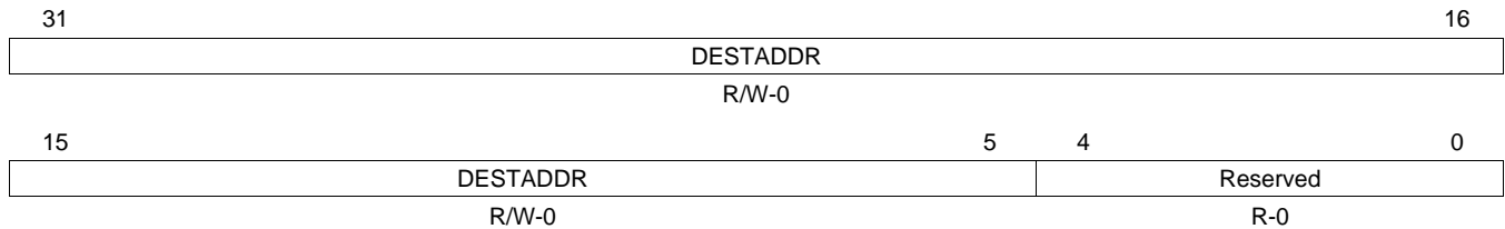
Figure 5-7. IDMA Channel 0 Destination Address Register (IDMA0_DEST)
