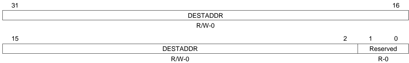
Figure 5-11. IDMA Channel 1 Destination Address Register (IDMA1_DEST)
