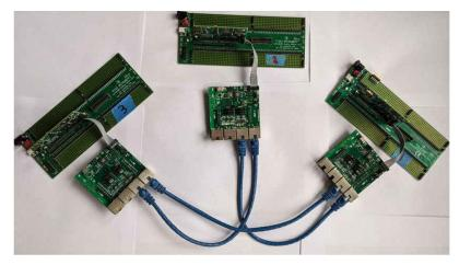
Figure 5-5. Test Platform for Three Devices Communication
