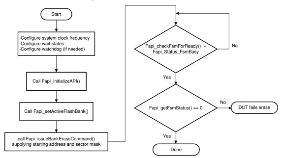
Figure 4-2. Recommended Bank Erase Flow
