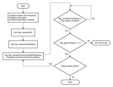
Figure 4-1. Recommended Erase Flow
