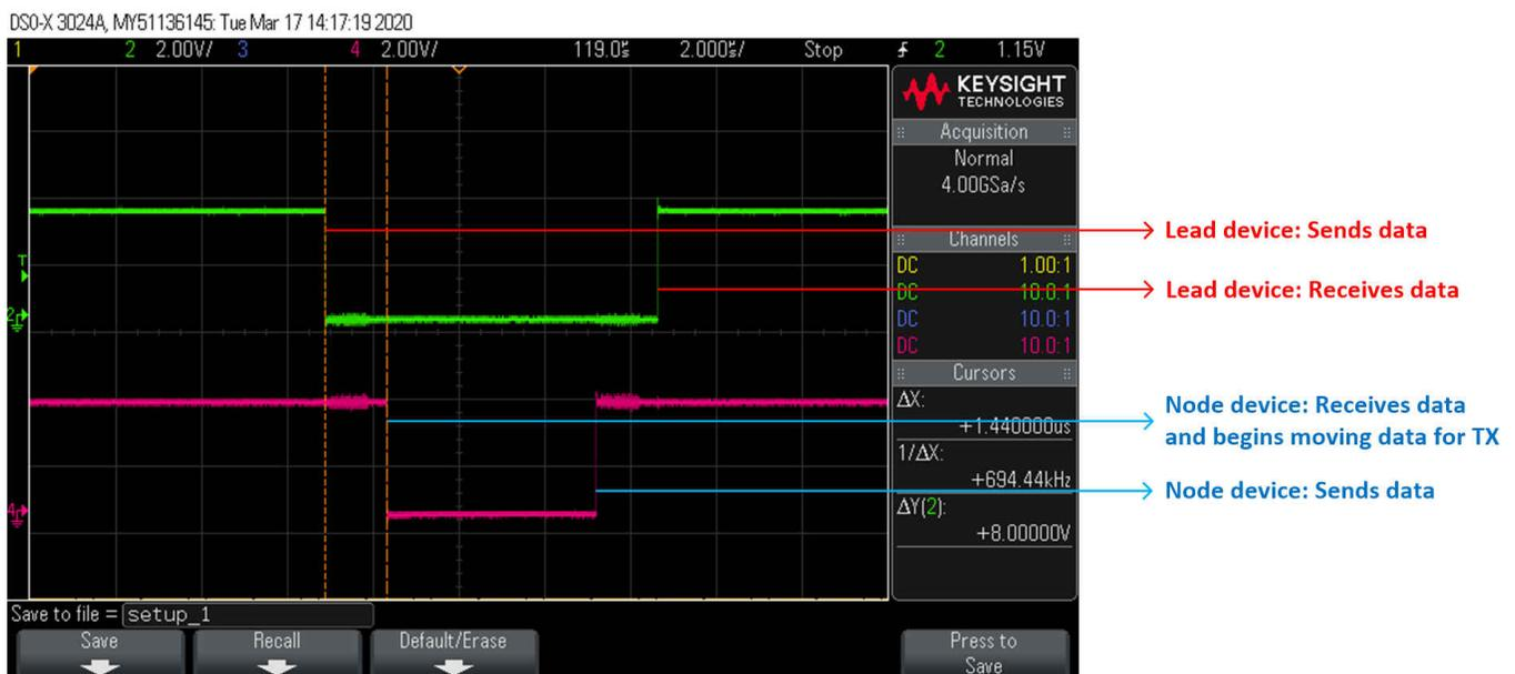
Figure 5-3. Data Transmission Test Using CPU Control
