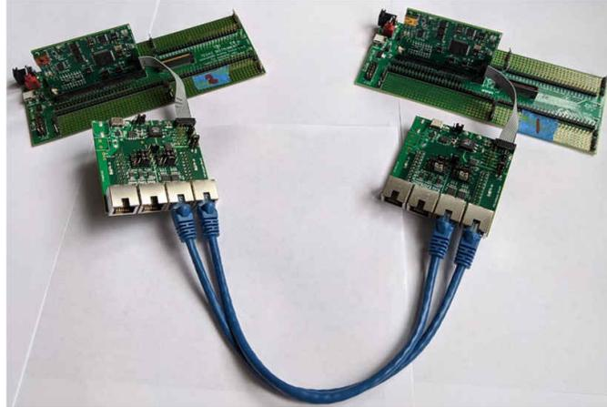
Figure 5-2. Test Platform for Two Device Communication
