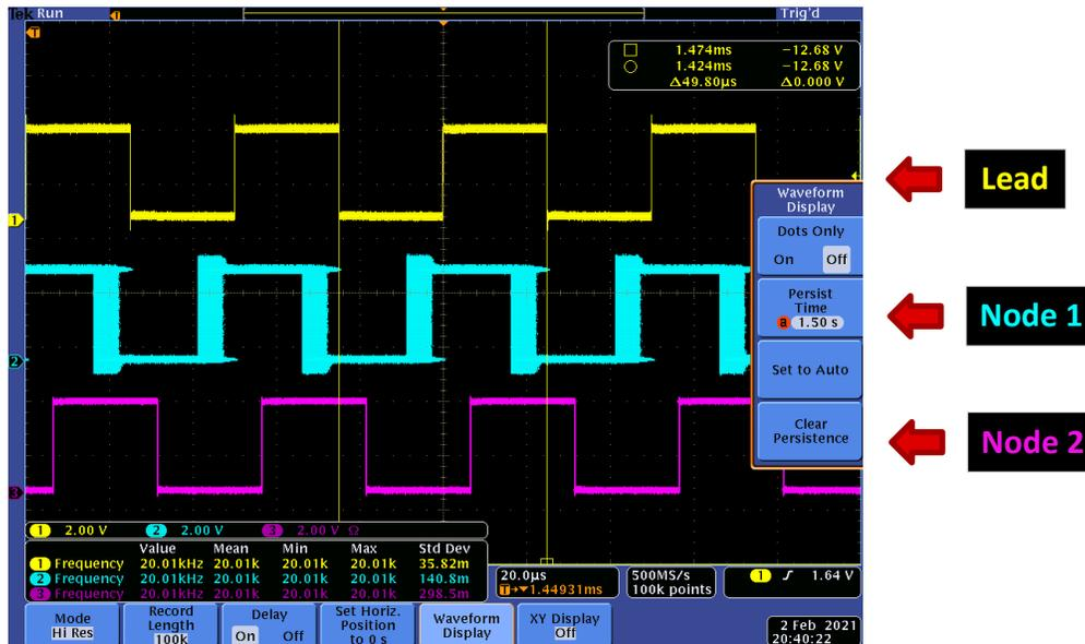
Figure 7-9. 1 Lead - 2 Node Device without EPWM Synchronization
