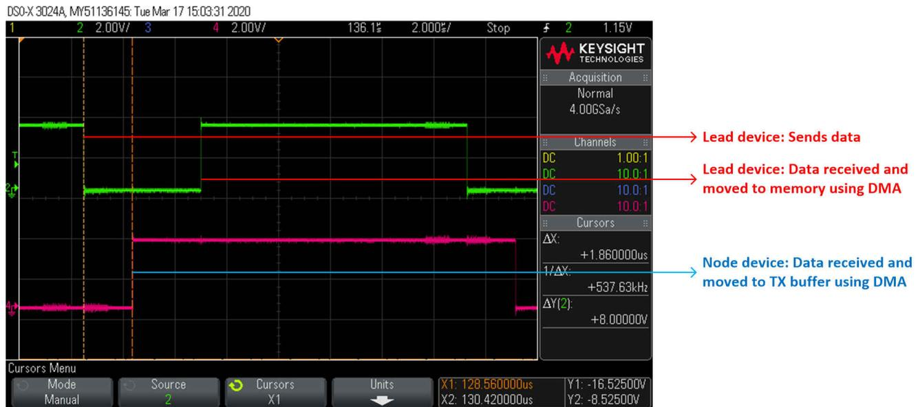
Figure 5-4. FSI Communication Using DMA Control
