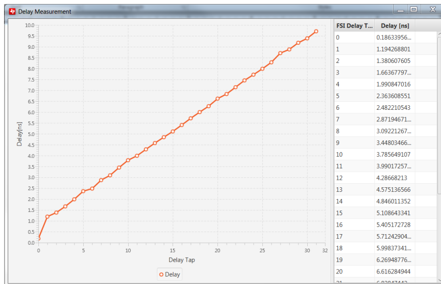
Figure 8. FSI Skew Compensation Utility - Delay Measurement
