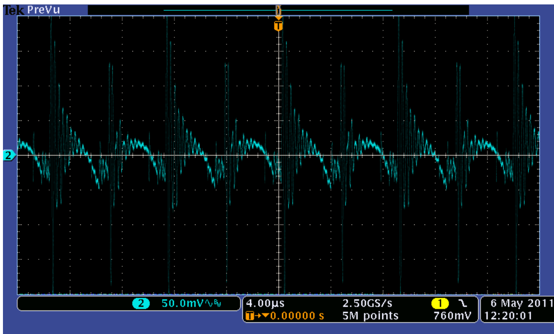
Figure 30. High Frequency Voltage Ripple (Blue – Output Voltage)
