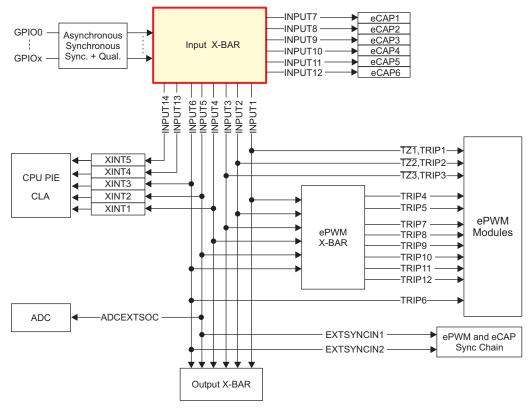
Figure 2. Input X-BAR
