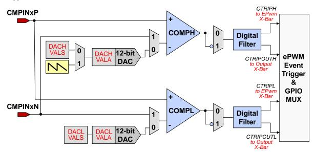
Figure 1. Comparator Subsystem (CMPSS) Block Diagram
