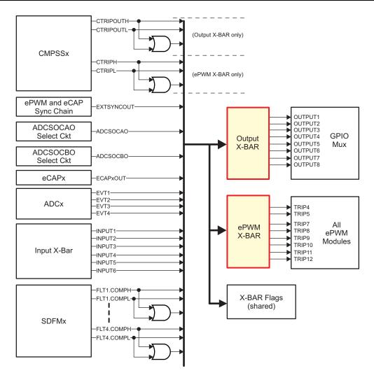
Figure 3. Output and ePWM X-BARs
