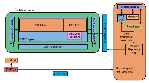
Figure 2. HWBIST In-System Block Diagram
