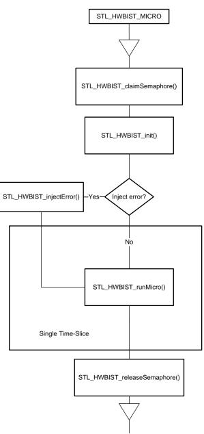
Figure 5. Flow Chart of Time-Sliced Micro-Run Execution
