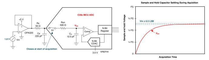
Figure 1-1. Settling of the ADC S+H Capacitor
