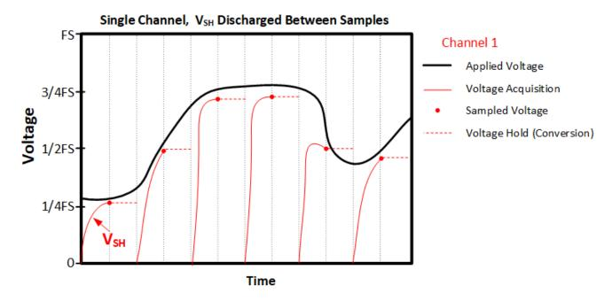
Figure 1-3. Sequence of Samples With C<sub>H</sub> Discharged Between Conversions
