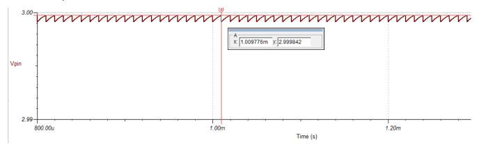
Figure 4-2.  $C_s$  Voltage With  $R_s$  = 100  $\Omega$
