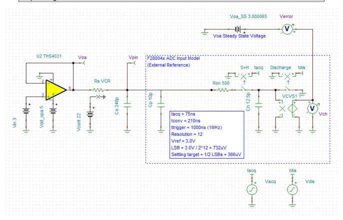
Figure 2-2. F28004x ADC Input Model
