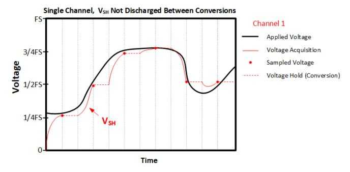
Figure 1-2. Sequence of Samples With CH Retained Between Conversions
