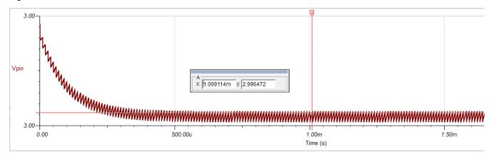
Figure 4-3.  $C_s$  Voltage With  $R_s$  = 1k  $\Omega$
