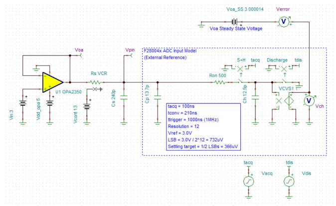
Figure 3-2. F280049 Example TINA-TI Circuit
