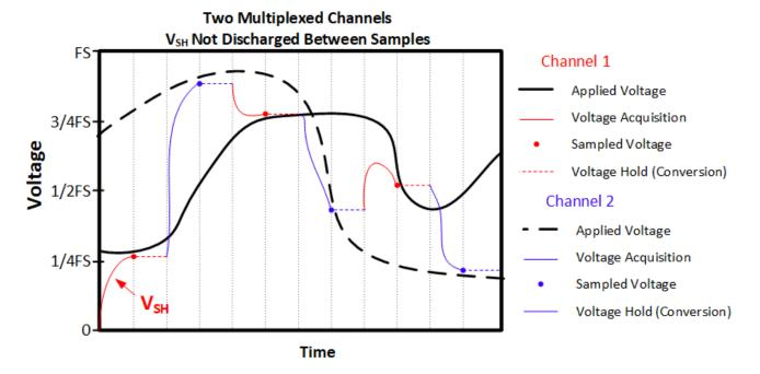
Figure 1-4. Sequence of Multiplexed Samples
