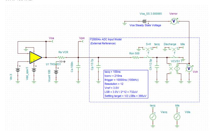
Figure 4-1. Example Circuit Utilizing Charge Sharing
