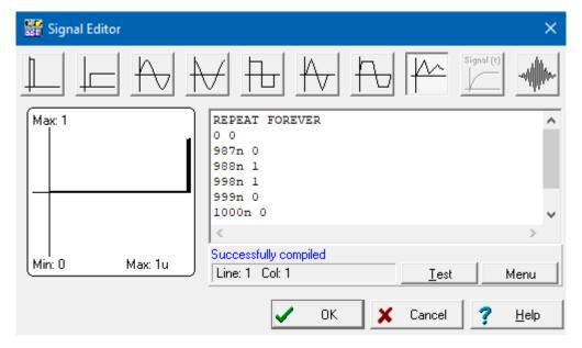
Figure 2-4. Example Timings for t<sub>dis</sub> (Piecewise Linear)
