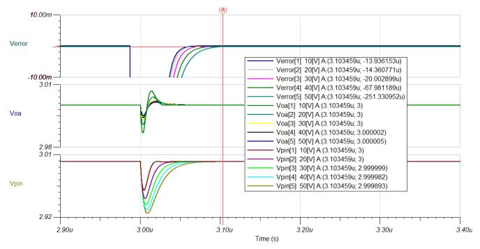
Figure 3-10. F280049 Example R<sub>s</sub> Fine Sweep Results
