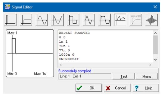
Figure 2-3. Example Timings for t<sub>acq</sub> (Piecewise Linear)
