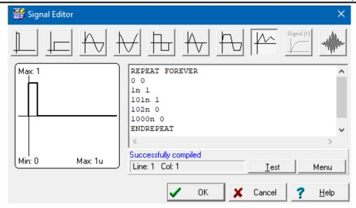
Figure 3-3. F280049 Example T<sub>acq</sub> Source Timings
