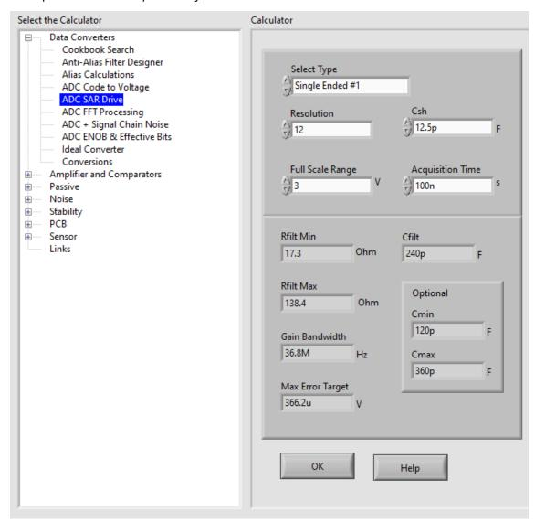
Figure 3-1. F280049 Example Analog Engineer's Calculator Output
