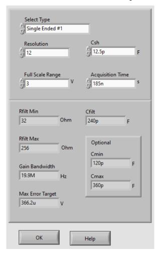
Figure 4-4. Analog Engineer's Calculator Output for OPA2320
