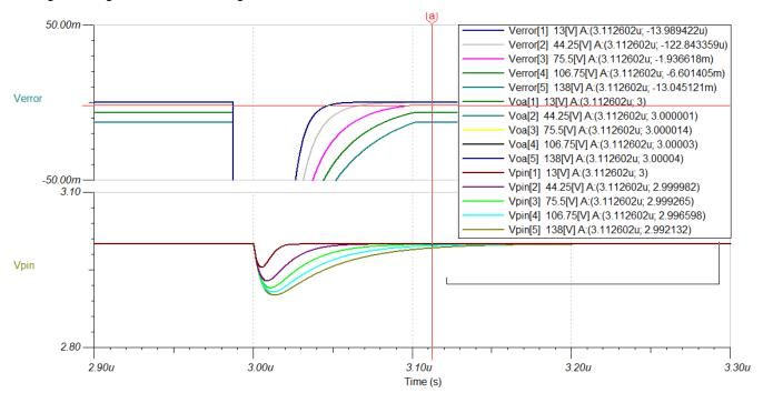
Figure 3-9. F280049 Example R<sub>s</sub> Initial Sweep Results
