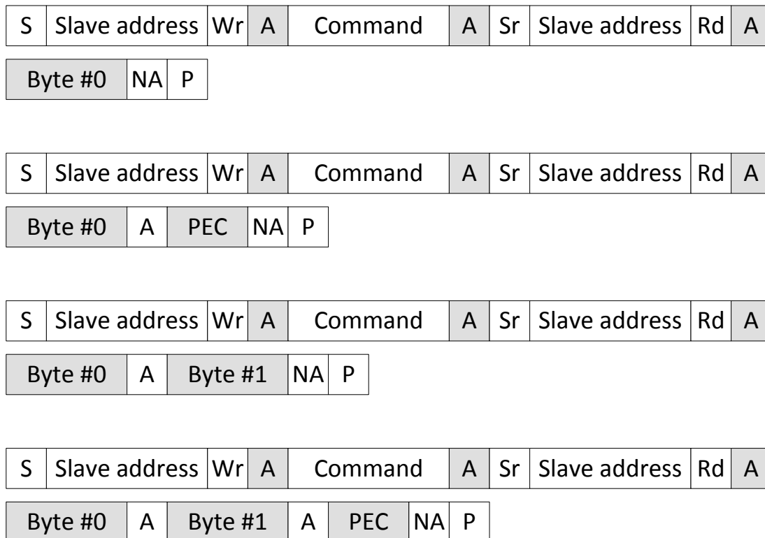
Figure 35-6. Read Byte and Read Word Messages With and Without PEC
