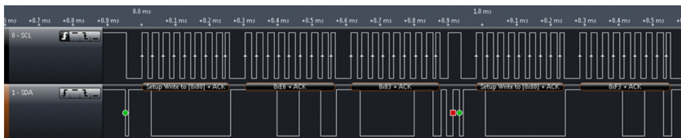
Figure 18. I2C Set Up and Start Temperature Measurement
