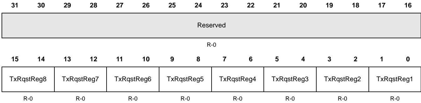
Figure 10-30. Transmission Request X Register (DCAN TXRQ X) [offset = 0x84]
