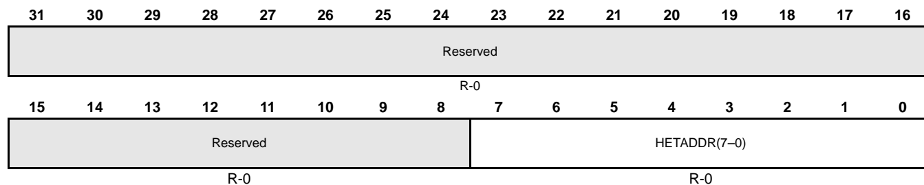
Figure 12-38. HET Current Address Register (HETADDR) [offset = 0x08]
