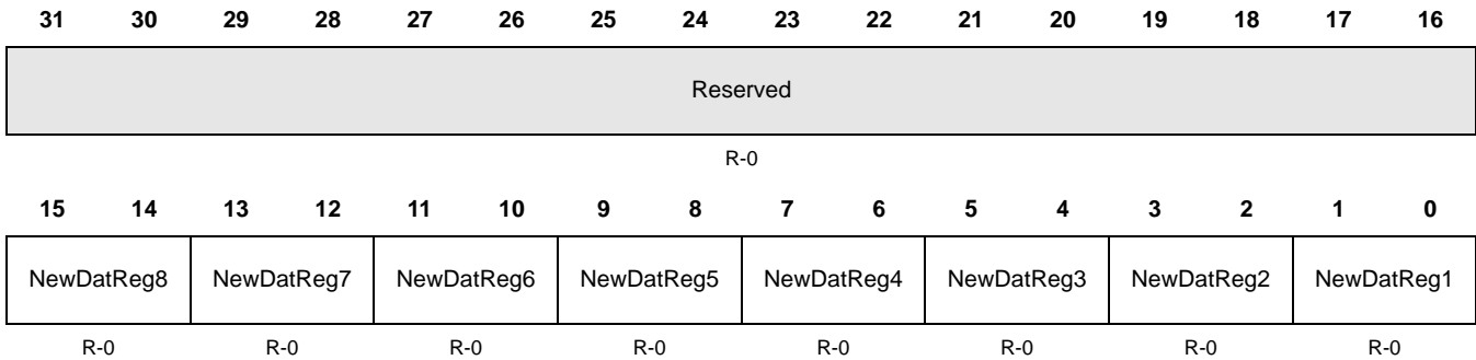
Figure 10-32. New Data X Register (DCAN NWDAT X) [offset = 0x98]
