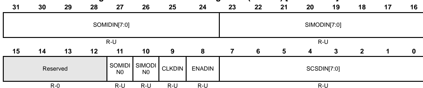
Figure 11-8. SPI Pin Control Register 2 (SPIPC2) [offset = 1Ch]
