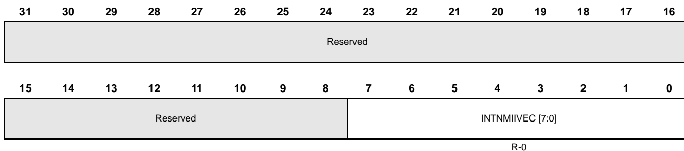
Figure 8-11. NMI Index Offset Vector Register (INTNMIIVEC)
