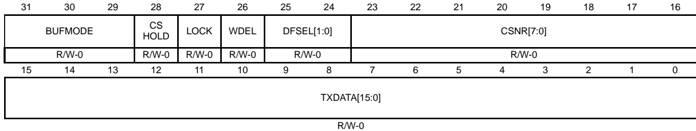
Figure 11-49. Multi-buffer RAM Transmit Data Register [offset = Base + 000–1FFh]
