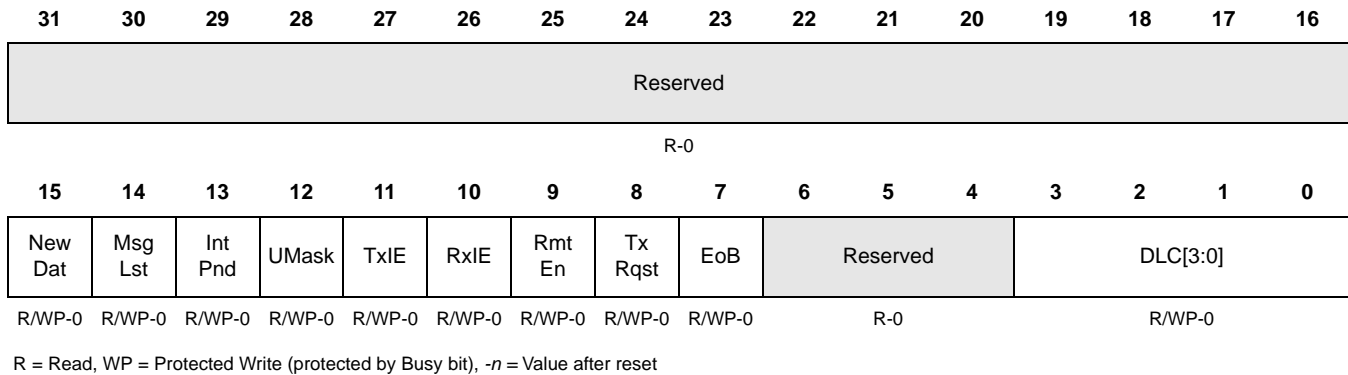
Figure 10-46. IF2 Message Control Register (DCAN IF2MCTL) [offset = 0x12C]
