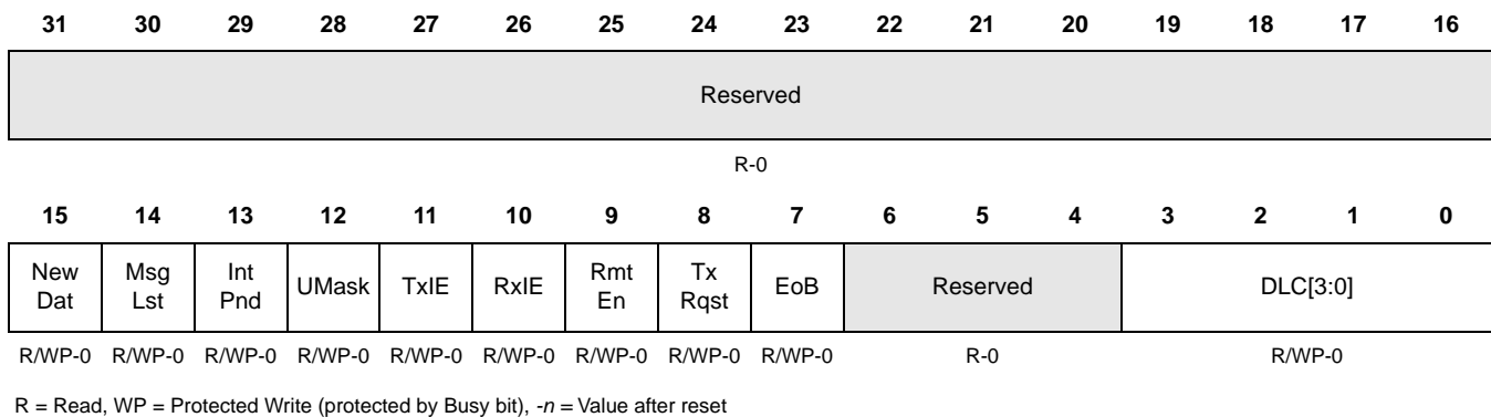
Figure 10-46. IF2 Message Control Register (DCAN IF2MCTL) [offset = 0x12C]
