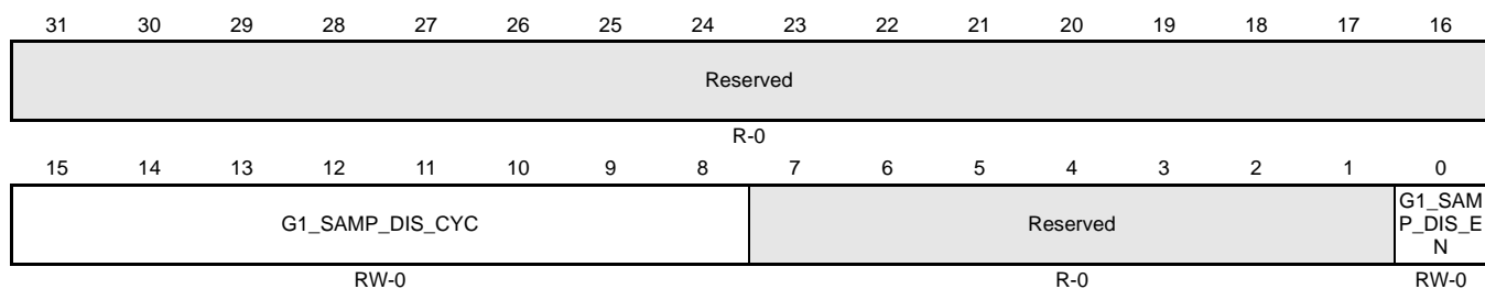
Figure 15-63. ADC Group1 Sample Cap Discharge Control Register (ADG1SAMPDISEN) [offset = 0x120]
