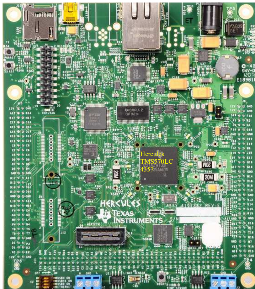
Figure 2-1. TMS570LC43 HDK Board, Interfaces Top Side
