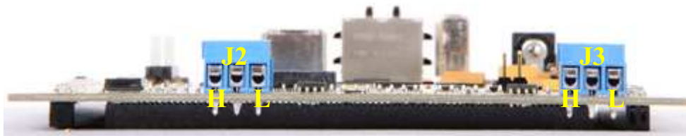
Figure 2-4. J2, J3 CAN Bus Interface (Screw Terminal)
