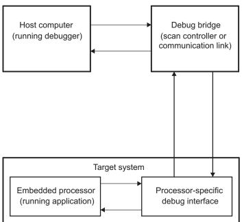
Figure 1-1. Debugging an Embedded Processor
