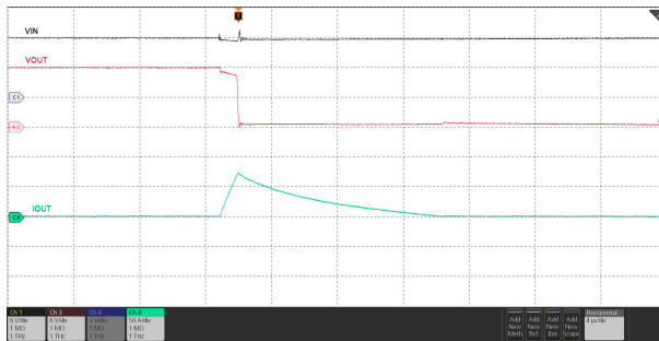
Figure 8-10. Output Short-Circuit During Steady-State
