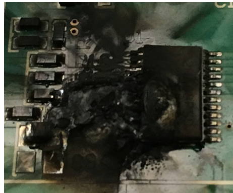
Figure 2. Thermal Damage Caused by an Overcurrent Event
