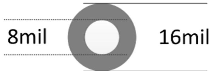
Figure 11-6. Recommended Minimum Via Sizing
