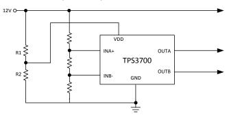
Figure 1. Voltage Divider at VDD
