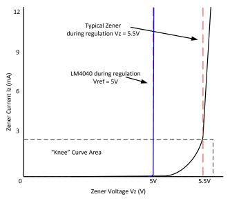
Figure 3. Zener Diode I-V Reserve Voltage characteristics
