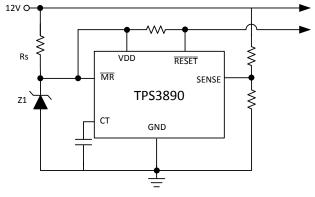
Figure 2. Zener Diode at VDD
