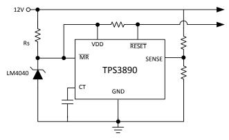
Figure 4. LM4040 at VDD
