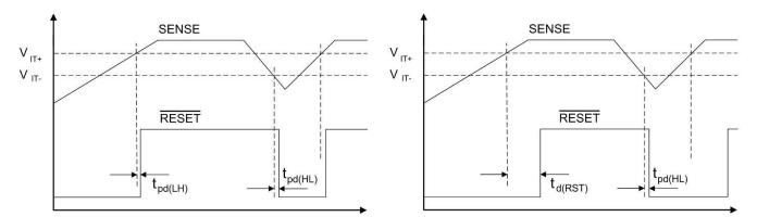
Figure 1. Voltage Detector (Left) vs Voltage Supervisor (Right)
