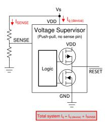
Figure 9. Push-Pull, Sense Pin, Voltage Supervisor
