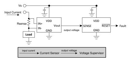
Figure 4. Using a Voltage Supervisor for Current Sense Fault Protection
