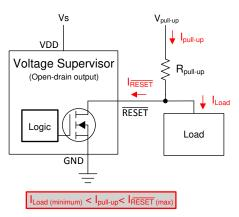
Figure 13. Calculating Pull-Up Resistor for Open-Drain Outputs
