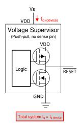
Figure 8. Push-Pull, No Sense Pin, Voltage Supervisor
