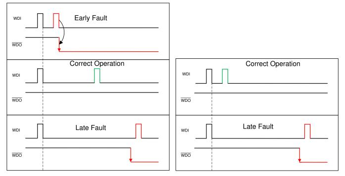
Figure 11. Window (Left) vs Standard (Right) Watchdog Timers
