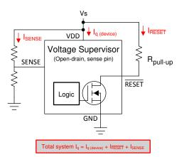
Figure 7. Open-Drain, Sense Pin, Voltage Supervisor
