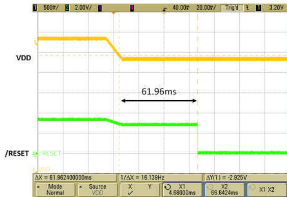
Figure 9-3. Sense Delay where CTS = 0.1 μF
