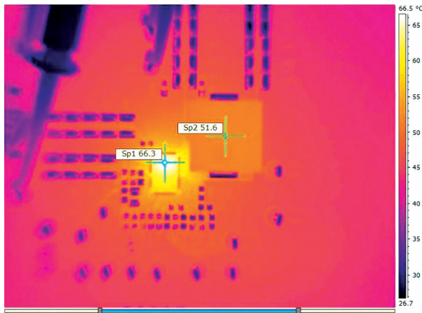
Figure 5. TPS548B22 thermal performance, T_{max} = 66.3^{\circ}\text{C} .
