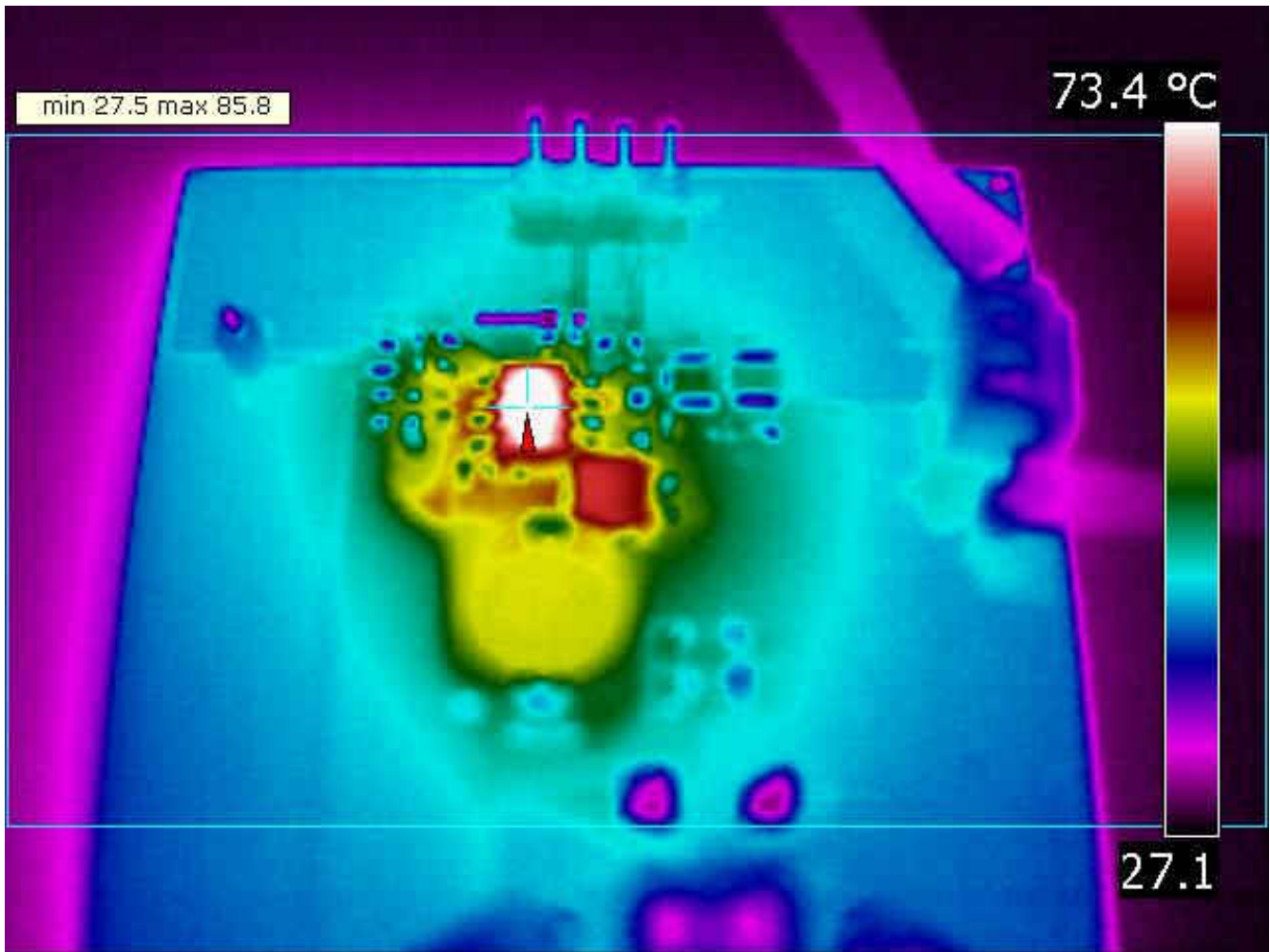
Figure 2-12. TPS54231EVM-372 Thermal Image
