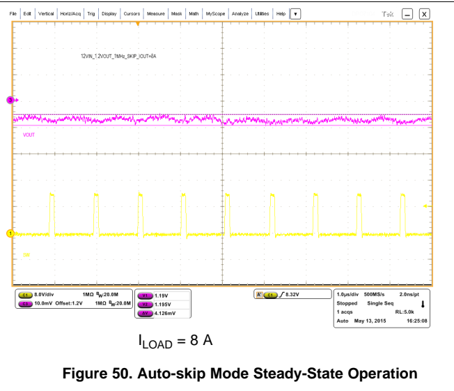
Figure 48. Auto-skip Mode Steady-State Operation
