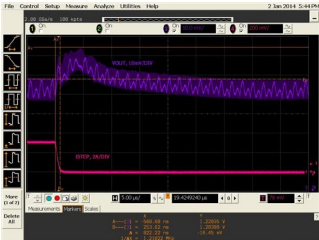
Figure 4-2. Step-Down Load Transient Response
