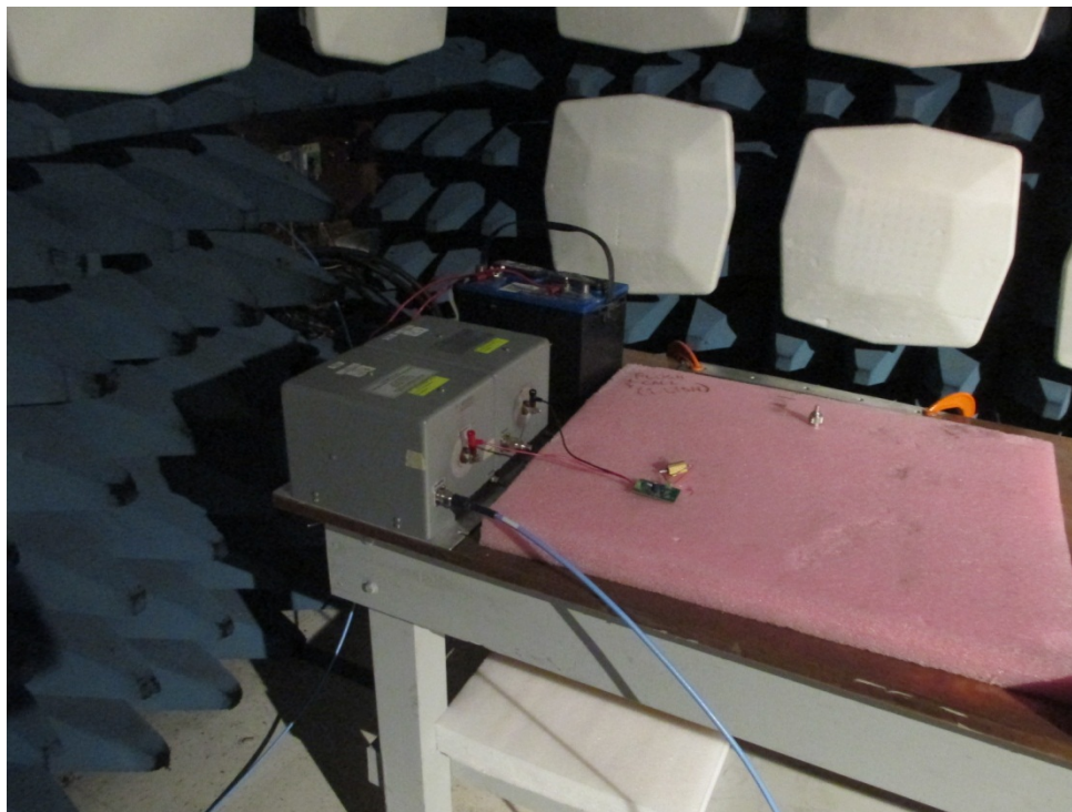
Figure 1. Setup for Conducted Emission (CE) Measurements
