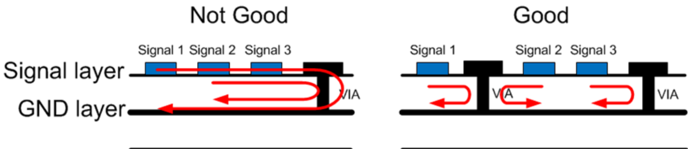
Figure 11. Localizing Noise Source to Form Smaller Current Loops
