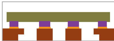
HotRod™ interconnect (flip-chip-on-lead) QFN
