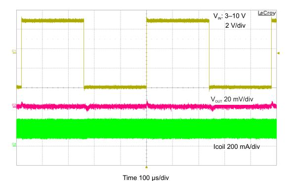
Figure 24. Line Transient Response with 120-mA Load
