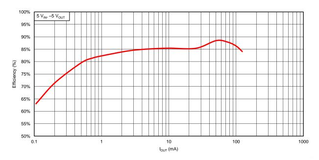
Figure 17. Efficiency versus Load Current with V<sub>OUT</sub> = −5 V
