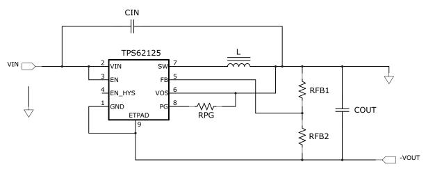
Figure 2. TPS62125 Inverting Buck-Boost Topology
