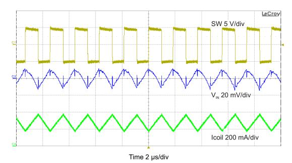
Figure 21. Input Voltage Ripple with  $V_{\rm IN}$  = 5 V and 120-mA Load
