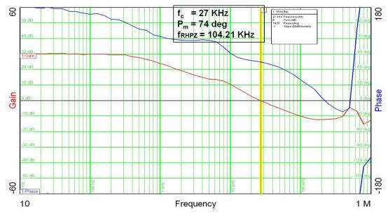
Figure 15. Bode Plot with  $V_{IN} = 5 \text{ V}$  and 120-mA Load
