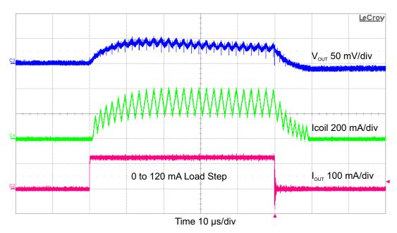
Figure 20. Load Transient Response with  $V_{\rm IN}$  = 5 V
