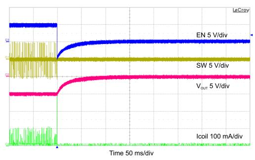
Figure 12. Shutdown at No Load and PG Pin Discharge of 100 Ohm
