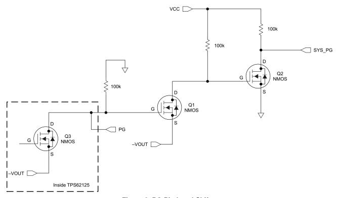
Figure 8. PG Pin Level Shifter
