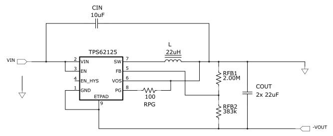
Figure 16. Schematic of the Tested Circuit
