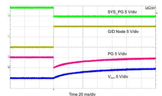
Figure 10. PG Pin Level Shifter on Shutdown
