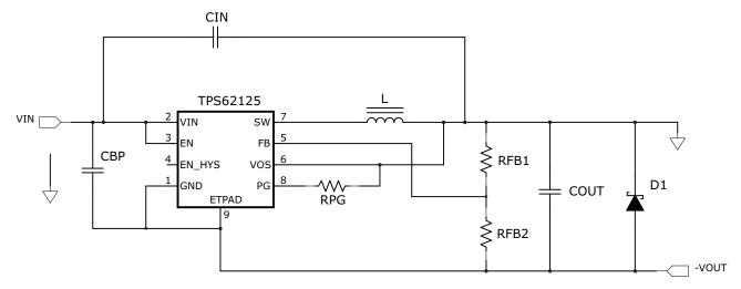
Figure 14. If Installing CBP, Installing Schottky D1 is Required
