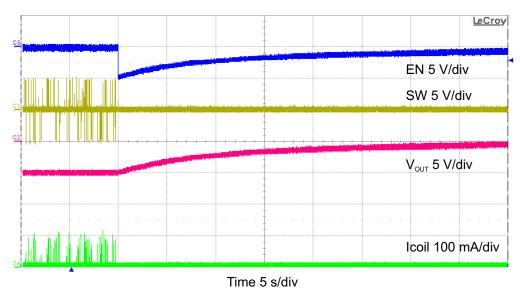
Figure 11. Shutdown at No Load and No PG Pin Discharge
