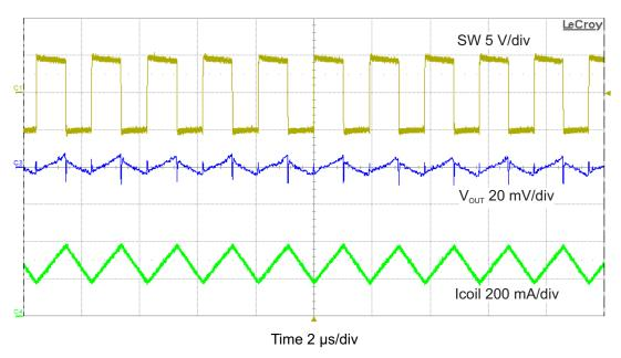
Figure 22. Output Voltage Ripple with  $V_{\rm IN}$  = 5 V and 120-mA Load
