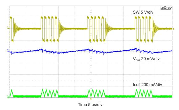
Figure 23. Output Voltage Ripple with  $V_{IN} = 5 \text{ V}$  and 10-mA Load
