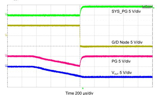
Figure 9. PG Pin Level Shifter on Startup
