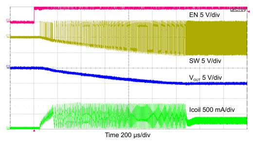
Figure 13. Startup Behavior in the Inverting Configuration with  $V_{IN} = 5$  V and 120-mA load
