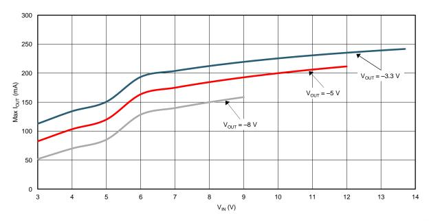
Figure 4. Maximum Output Current versus Input Voltage
