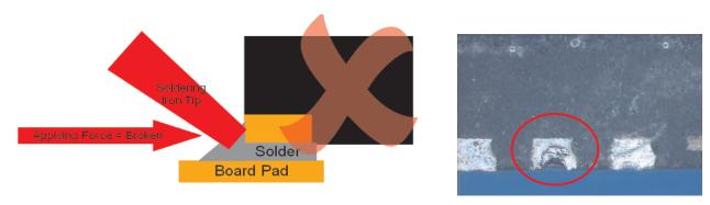
Figure 18. Manual Rework Damage
